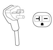
240V / 20 Amps Electrical Circuit Required NEMA 6-20p
