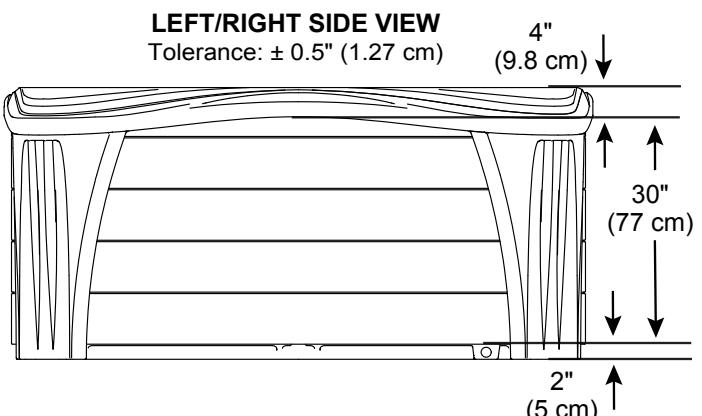
**IMPORTANT!** Always measure each hot tub for exact dimensions BEFORE designing its foundational support and/or decking.
